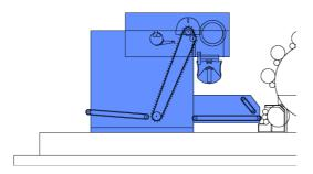
The automatic hopper feeder introduces the raw material in the carding machine in a regular and constant way.
