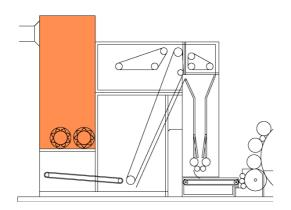
The silo receives the raw material from pipes coming form the blending plant (pipes are excluded from our quotation) and feeds the automatic volumetric feeder.
