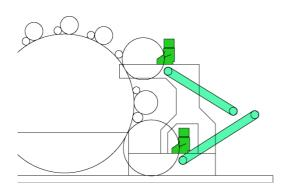
The fly combs detach the web from doffer rollers, then the belt conveyors transport it to the following unit. The webs union permits a better regularity of the final product.
