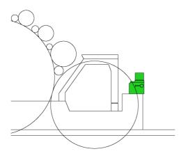
The fly comb detaches the web from doffer roller and send it to the next unit. The fly comb moves at high speed with a 40 mm oscillation.
