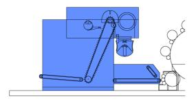
The automatic hopper feeder introduces the raw material in the carding machine in a regular and constant way.
